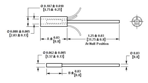
XS-B (Supplied with extension rod already attached to core)
