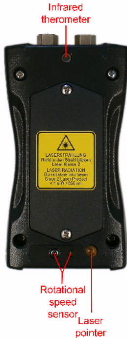
Figure 33: Rotation speed and temperature sensor, laser pointer
