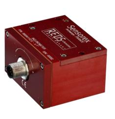
Meggitt (Sensorex) SX41100 high-performance analog/ digital servo-inclinometers provide an output signal proportional to the angle of measurement, with choice of  $\pm 5V$  analog or 4-20mA, and RS 232 or RS 485 digital outputs, and a maximum linearity error specification of less than  $\pm 0.02\%$  FS as standard.
