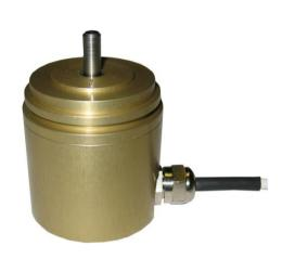
Meggitt (Sensorex) (IS) SX36RV provides a sinusoidal signal, with a linear voltage over the measurement range. The primary is excited by an AC voltage, and is picked up by the secondary winding on the transformer principle; the position of the rotating core determines the transformer ratio of each secondary winding.
