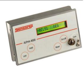
The Meggitt (Sensorex) SX42891 inclinometer is a self contained angle measuring unit with integrated display. With its own internal battery (2 x 1.5V AALR6) and LCD, the angle can be directly read either in degrees, mrads, and mm/m.
