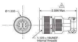
Length is with threads fully engaged.
