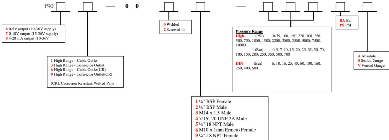
Examples : P9061-0002-7K5PSS = 0 to 5V output from 10 to 36V supply, cable outlet, welded 1/4" BSP male port, 7500 psi sealed gauge
