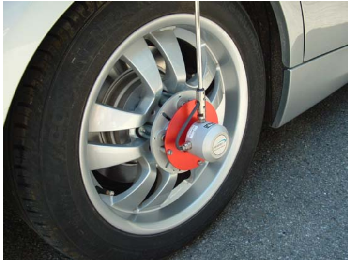
MT100/e KFZ-RS with PEISELER MOUNTING PLATE fitted to a car wheel
