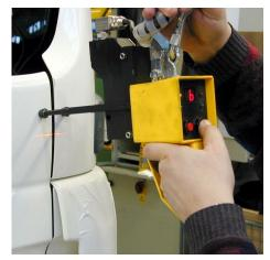
The M2D-75/30-LaserScanners have a range of 30 mm in x-axis, scann frequency is 50 Hz. The z-axis range is 75 mm, standoff distance is 90 mm. This allows to measure at at a distance, rubber feet protect the fresh paint car against damage.
