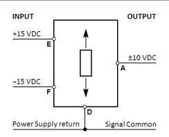
A through F: Connector pin assignments
