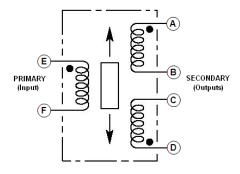
A through F: Connector pin assignments; Connect B to C for differential output
