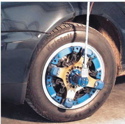
3: 6-component wheel force transducer with telemetric data transmission
