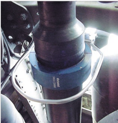
1: Torque measurement on a truck cardan shaft
