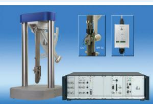
**CS18 LS**, system with shock pendulum for calibrating sensors at low shock acceleration up to 200 g<sub>n</sub>. Efficient system for calibrating crash sensors up to a mass of 300 gram
