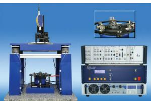
**CS18P HF**, System for the absolute method of vibration calibration in frequency range 5 Hz to 20 kHz
