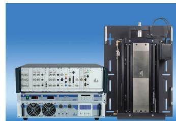
**CS18 VLF System** for the comparison calibration of vibration sensors at very low frequencies 0.2 Hz to 160 Hz, e.g. seismic sensors with a weight of up to 3 Kilogram and sensors of whole-body vibration
