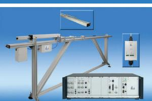
**CS18 HS**, system for calibration of sensors with high shock acceleration up to 100.000 g<sub>n</sub>. Efficient system for calibrating shock sensors
