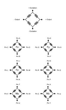
Bridges Fz; Mz = 700 ohms Bridges Fx; Fy; Mx; My; = 350 ohms **Connector Type:** Souriau 851-02E16-26P50-44
