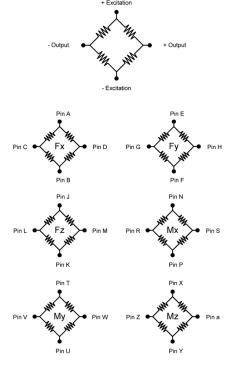
Bridge Fz = 700 ohms Bridges Fx; Fy; Mx; My; Mz = 350 ohms Connector Type: Souriau 851-02E16-26P50-44
