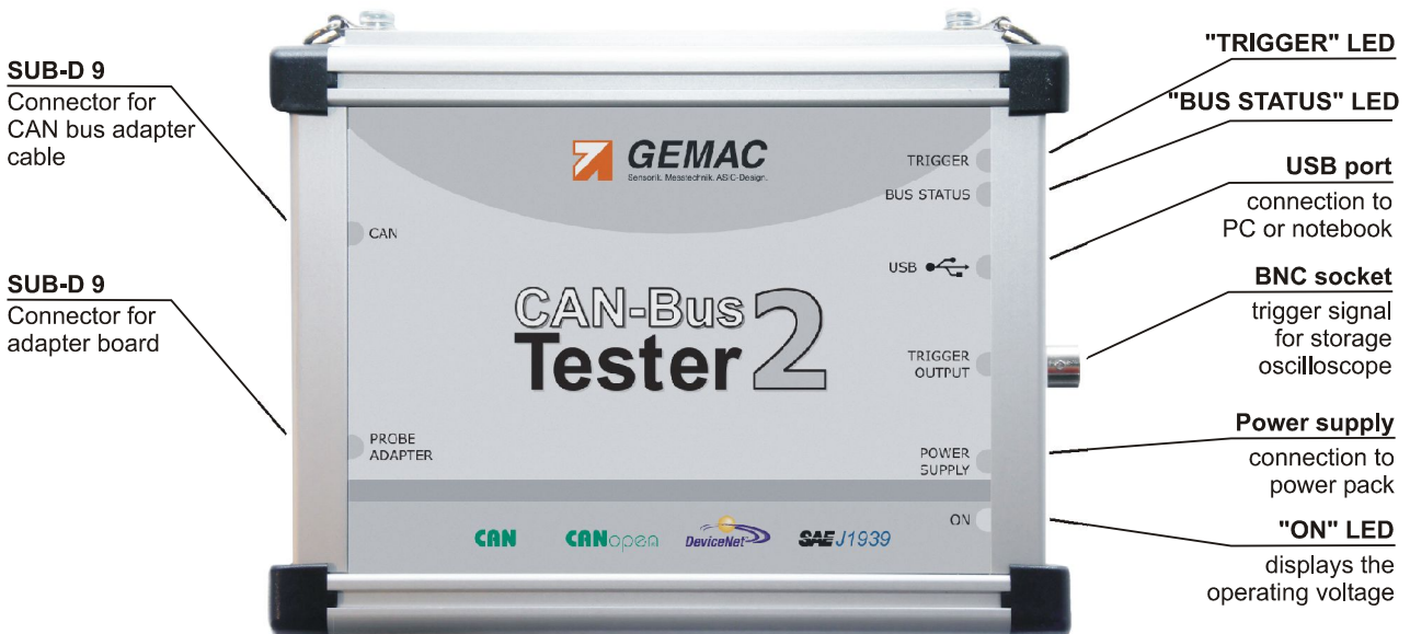
Figure 1: Connections of the CBT2
