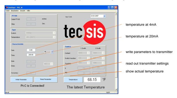
In order to set the measuring range, the plug connector must be removed and the measuring insert has to be taken out of the housing. After that the USB connection from PC to the interface on the board must be established. A detailed description, how to program the thermometer is given in the instruction manual.
