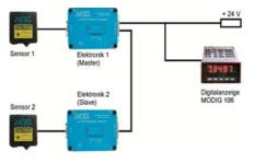
Cabling of thickness and differentiation measurement system with one sensor pair
