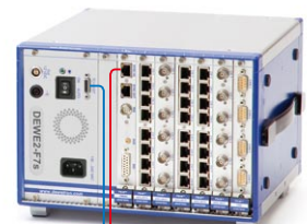
DEWE2-F7s with TRION-TIMING module
