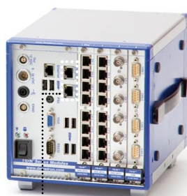
DW2-LAN-2 DEWE2-M4s with 2x 1 Gbit Ethernet option
