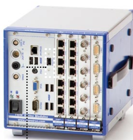
DW2-FIREWIRE-1 DEWE2-M4s with FireWire® option
